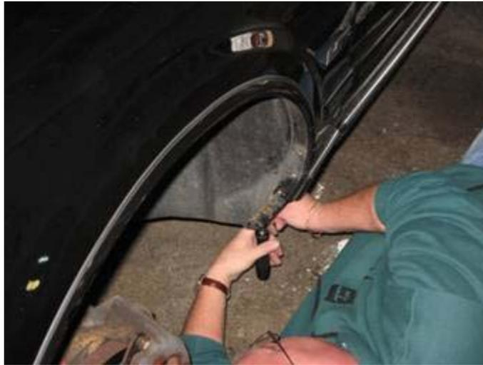
**CAREFULLY** remove the inner fender. It'll take just a bit of coaxing but it will come out:
