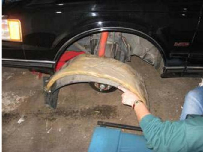
Now, when you look up into the fender well, you'll see a small plastic clip that holds the hood release cable to the inner body. That needs to be removed.
