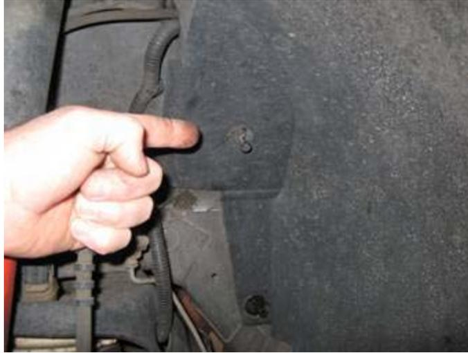
The next step is to remove the screws that hold the wheel well trim:
