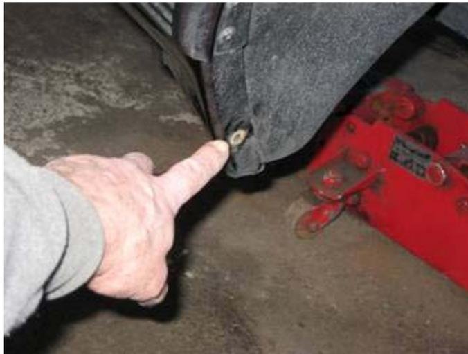
There are two more screws that need to be removed and they are located directly under the front edge of the door:
