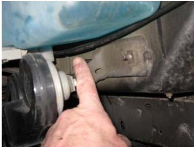
Then route the cable under the washer fluid reservoir remembering to replace the clip on the cable and attaching it back onto the inner body.
