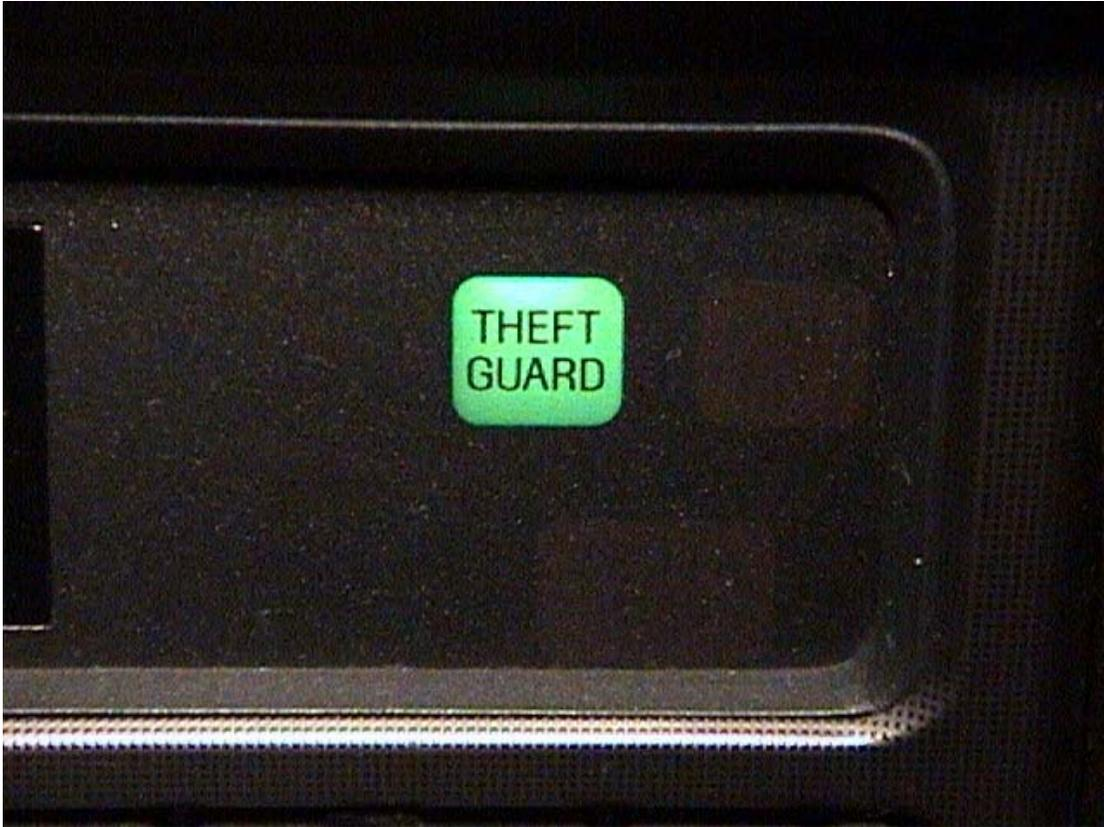
**Anti-Theft System** – This optional system helps protect your vehicle against break-ins or theft by monitoring all doors and the trunk lock cylinder.
